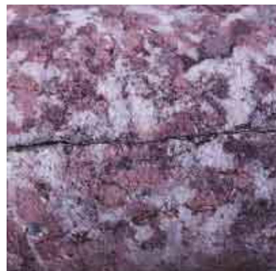
Granite drill core with natural fracture
