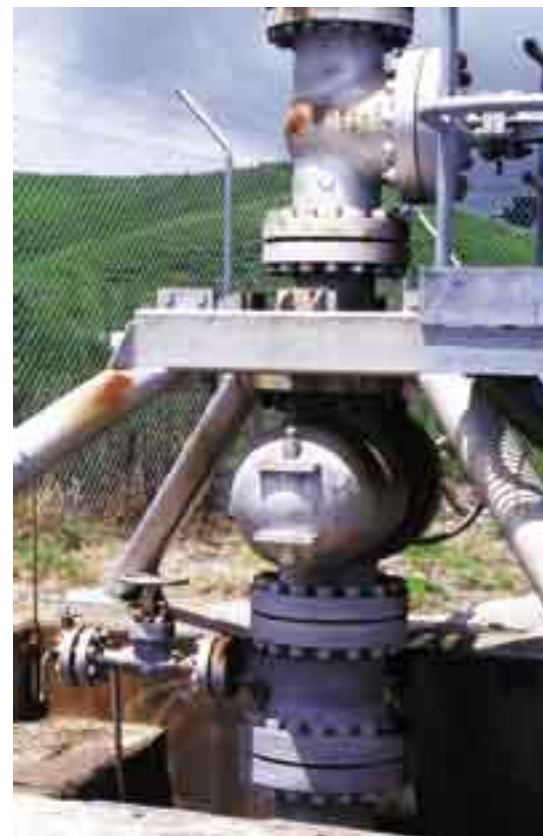
Geothermal well-head
